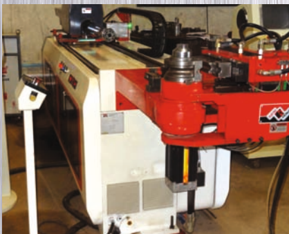
CNC Pipe Bending
